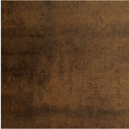
ME:01: Bronze aluminium to balustrade battens, canopy battens and canopy columns
